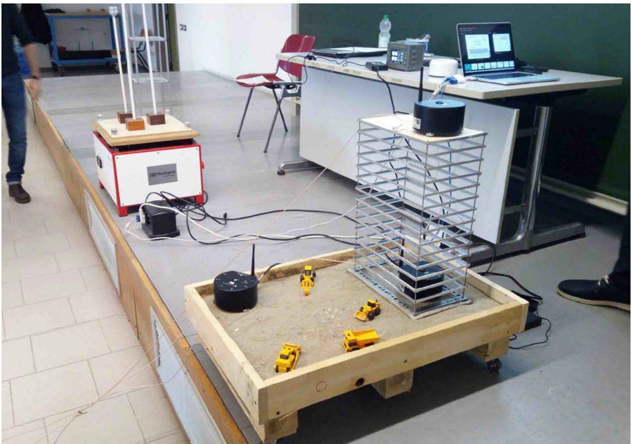
Tests on vibrating table simulating the seismic response of a building.
